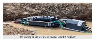
The ROBOMINERS prototype boasts a wide array of functions, including navigation, perception, excavation, material transport, and in-line material analysis. Rigorous experiments have yielded detailed insights into the technology's suitability for varying rock conditions, resulting in significant enhancements in its excavation performance.
