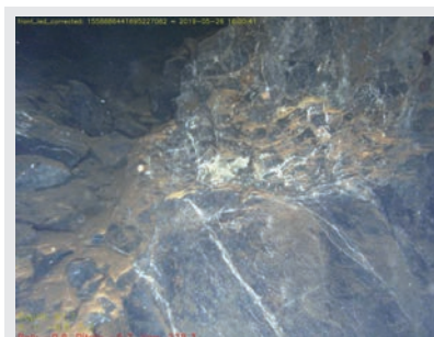
Edge of worked out pipe with calcite vein and chalcopyrite mineralization in limestone wall rocks.
