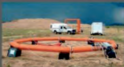
Receiver coil of 7.4 m in diameter measuring the vertical component of the magnetic field.
